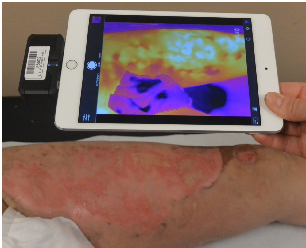
Figure 1. Thermography measurement with the thermal imager attached to an iPad mini.
